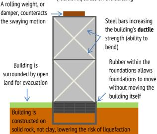
Ways in which buildings can be designed to reduce damage from an earthquake
